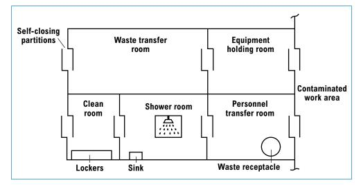
A decontamination facility consists of a shower room and a series of connected rooms separated by air locks.
