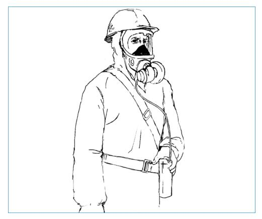
Workers can use full-facepiece PAPRs with P100 (HEPA) filters in asbestos concentrations up to 10 fibres per millilitre.
