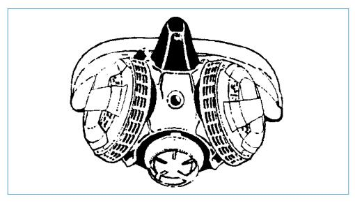
Workers can use half-facepiece, dual-cartridge respirators with P100 (HEPA) filters in asbestos concentrations up to 1 fibre per millilitre.
