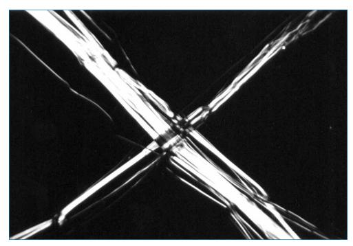
Asbestos fibres magnified many times.
